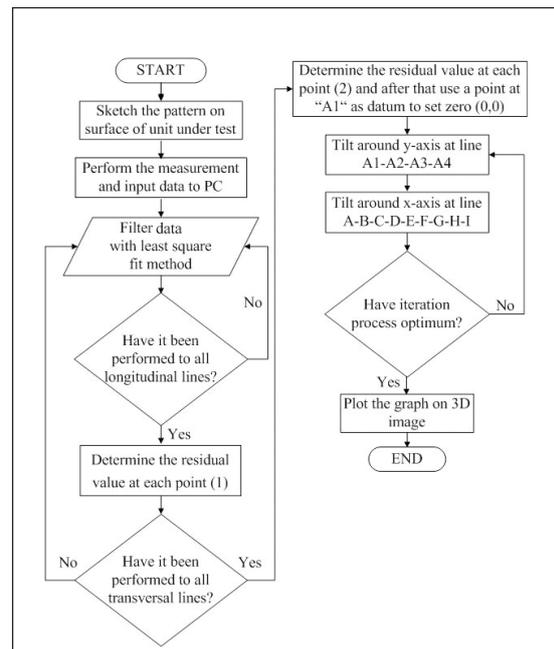
Figure 5. Measurement Procedure
