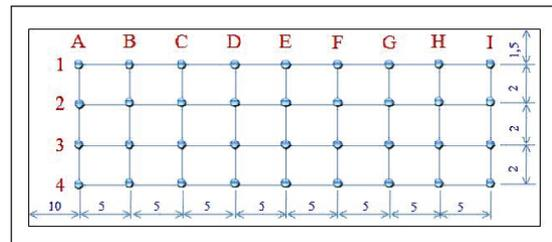
Figure 4. Pattern of Flatness Measurement (Distance in cm Unit)
