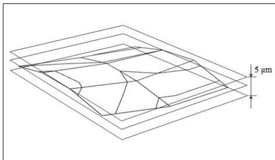
**Figure 1.** Illustration of Surface Flatness, i.e. 5  $\mu\text{m}$ .
