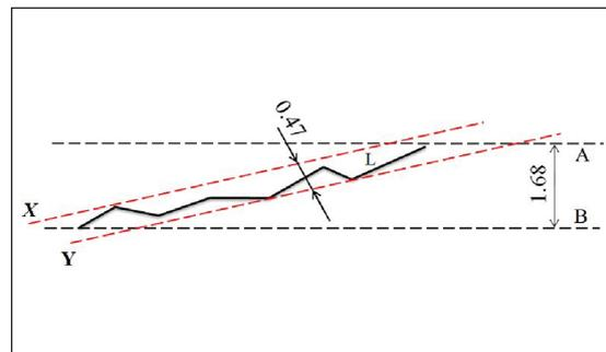
**Figure 2.** Example of Straightness Quality of a Line, i.e. 0,47 cm.
